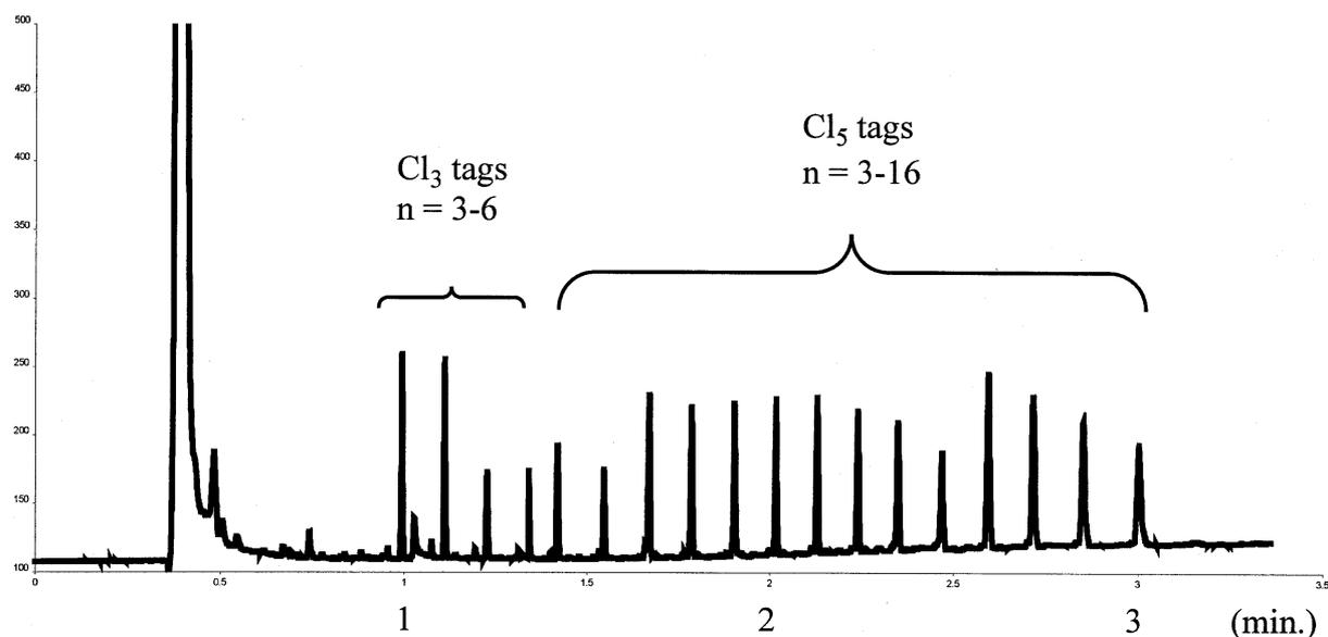
Figure 5. GC chromatogram of Cl<sub>3</sub> and Cl<sub>5</sub> tags on the HP 6890.
