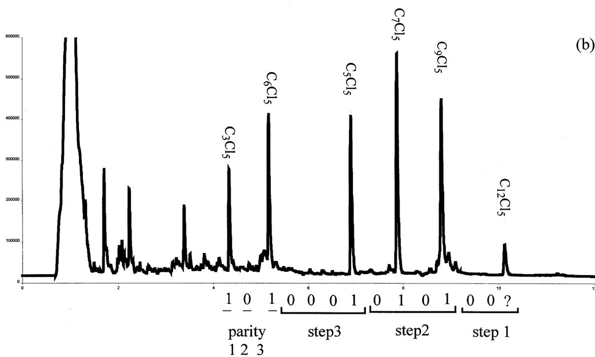
Figure 6. Rare events. When the GC/ECD auto score is ambiguous, parity tags are used to correctly identify tag signals [6]. (a) GC/ECD auto score of  $C_{10}Cl_5$  is incorrect. (b) GC/ECD auto score of  $C_{12}Cl_5$  is correct.
