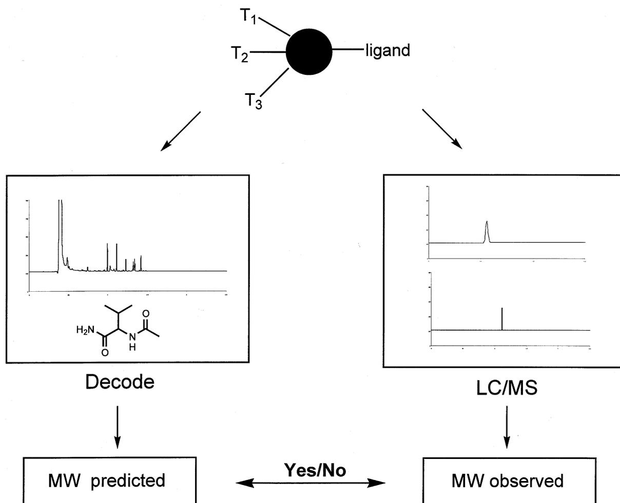
Figure 7. Schematic of decode-assisted, single bead LC/MS methodology.
