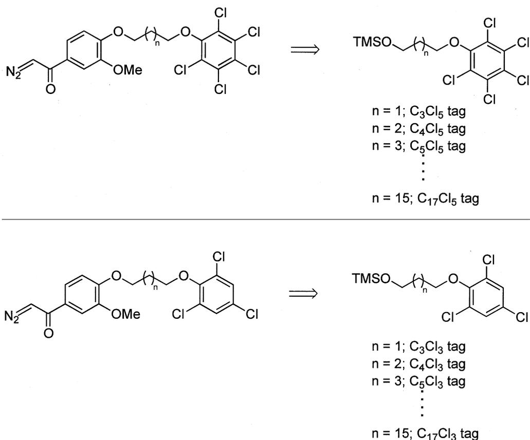
Figure 2. Structures of tagging molecules and corresponding trimethylsilyl ethers for GC/ECD analysis.
