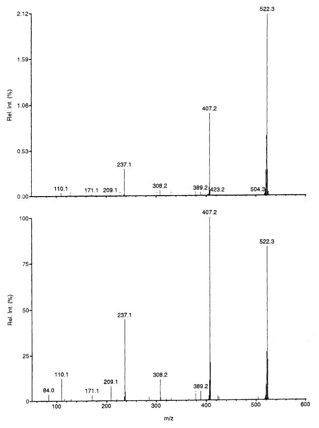
Figure 5. MS/MS of peak containing compound of molecular weight 522 (top) in comparison with the spectrum of resynthesized compound VIII (bottom).
