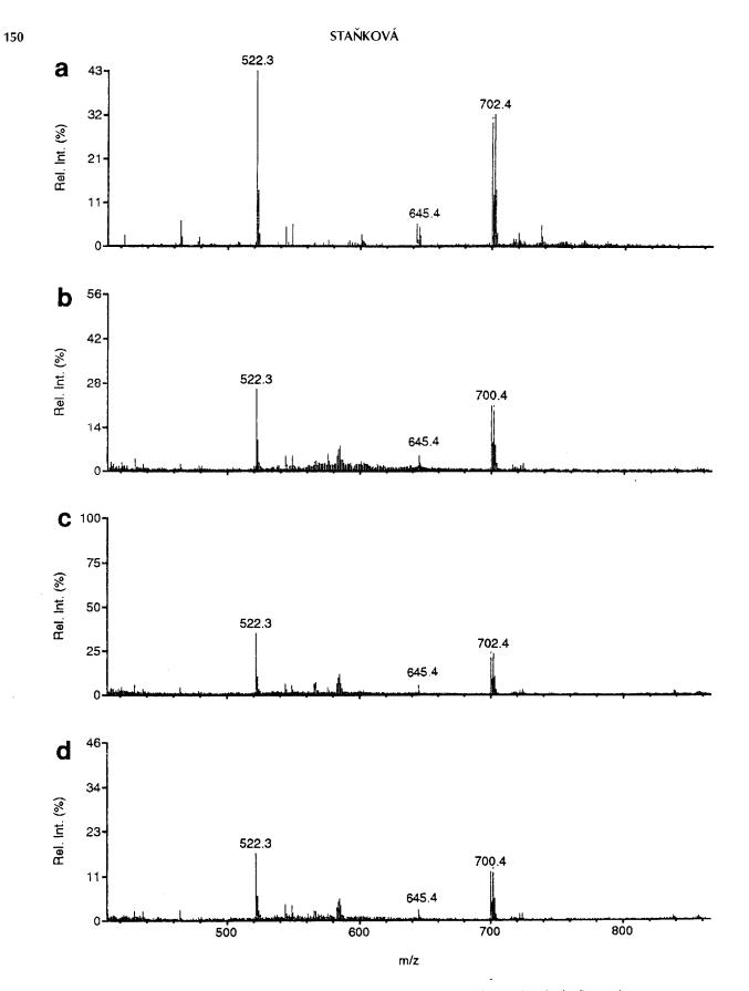
Figure 2. Mass spectra of compound mixture cleaved from three library beads (b–d) reacting positively with streptavidin compared with the mass spectrum of mixture cleaved from the beads synthesized using identified building blocks (histidine, trimethoxybenzaldehyde, and acetylglycine, a).
