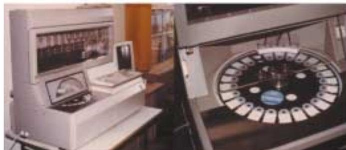
**Figure 2.** Centrifugal synthesizer for parallel synthesis of 24 peptides on cotton strips. Full view and detail of the rotor compartment.
