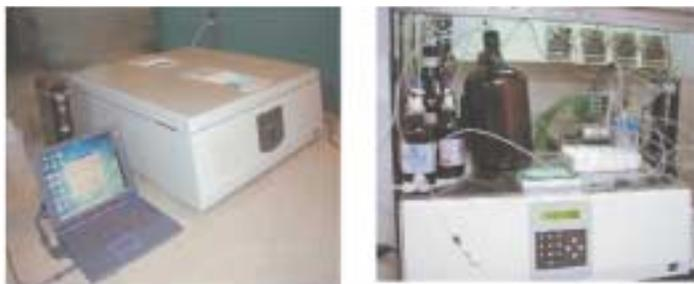
**Figure 7.** Commercially available (Spyder Instruments, Inc.) centrifugal synthesizer Compas 768 (on the left), and the same instrument modified for proof of concept oligonucleotide synthesis (on the right).
