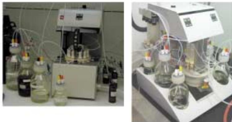
**Figure 10.** "Pet Oligator" - economical synthesizer capable of 24 parallel syntheses. On the left - one of the first prototypes. On the right - final version.
