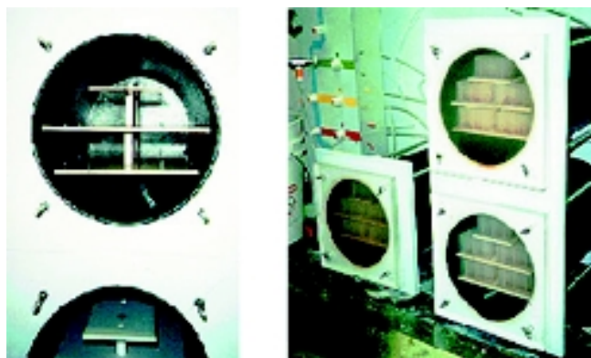
Figure 2 Polypropylene chambers used for cleavage of compounds from benzhydrylamine resin by exposure to gaseous HF. The window is made of polymethacrylate covered with polypropylene foil.
