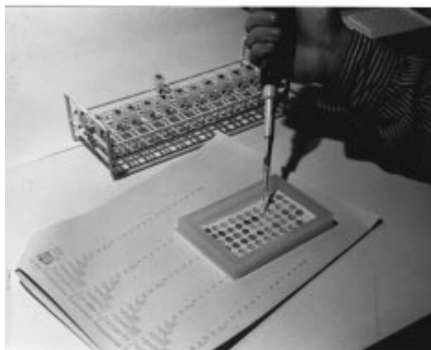
Figure 2. Simultaneous chemical synthesis on segmented, membrane-type solid support as developed at the GBF in Braunschweig, Germany. (A) The “filter disk method” of 1983 (with the hand of Helmut Blöcker). (B) The “SPOT synthesis method” of 1990 (with the hand of Sinan Güler).
